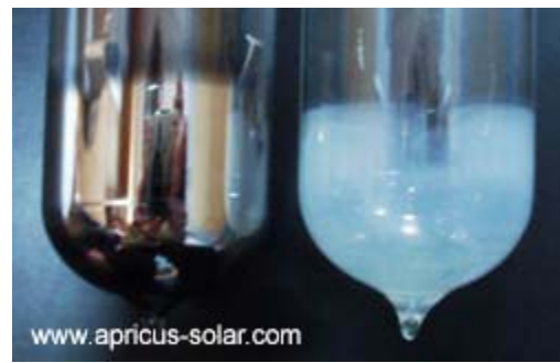
Left Tube = Vacuum Present Right Tube = Faulty
