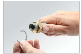
Slide on 1" union nut and close segment ring around pipe groove.
