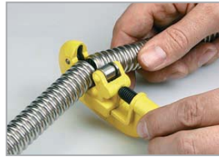
Cut pipe with tubing cutter. Do not use a hack saw.
